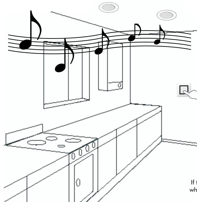
This function is designed for use in the event that the KB5OUND® power supply is fed by a specifically designated switch. In this case, the automatic activation mode must be programmed in order to automatically turn on the KB5OUND® unit when the switch is activated.
